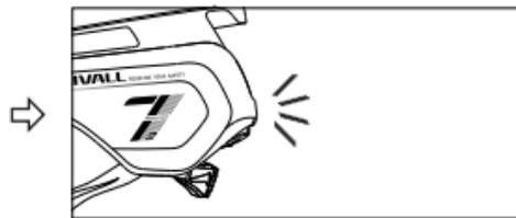
Then the tail light of the helmet will continue to flash in the light mode before connection. After connected successfully, the left turn signal or right turn signal can be realized by the BR80.
