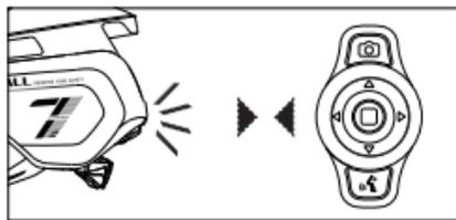
Put the power-on BR80 close to the main control of the helmet, and the warning light flashes three times per second, indicating that there is a BR80 that needs to be connected to the helmet.
