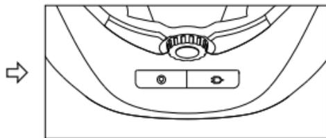
Press the power button of the helmet within 10s to confirm the connection of the BR80.
